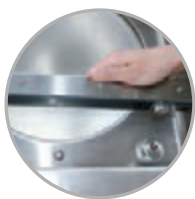
Barre saldanti estraibili Removable sealing bars
